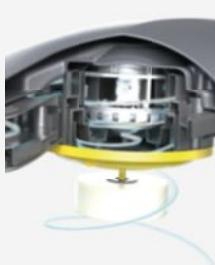
The TASKI ULTIMAXX range includes, as standard, patented TASKI whisper technology. This unique airflow system guarantees optimized suction and immediate noise absorption. With our unique cutting-edge technology the operation is extremely quiet with 63db(A) and with the eco mode it can reach as low as 60db(A). It is also available with HEPA filtration.
